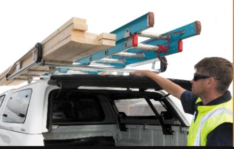
The versatile and adjustable configuration allows maxload to adapt to most common tub bodies, canopy heights and roof racks. The heavy duty uprights included in the maxload kit minimise chances of the canopy or tub cracking under pressure by providing a sturdy pillar of strength. Maxload allows users to maximise their vehicle's maximum carrying capability whilst avoiding costly damage, repairs or the prospect of a heavy load falling from the vehicle amidst traffic.
